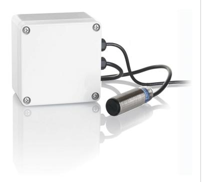
Developed with Dutch seed company Pop Vriend to monitor and optimise conveyor belt usage, this photoelectric sensor counts passing items in real-time at up to a meter distance. This sensor can detect and count transparent and reflective objects, and its visible, high power LED light compensates for dirt and makes alignment easy.
