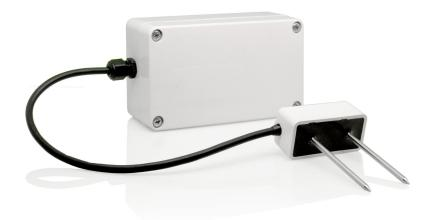
This soil sensor determines volumetric water content (VWC) by measuring the dielectric constant of the medium using capacitance and frequency domain technology to provide accurate measurements of all soils and soilless medias with a wide range of salinities.
