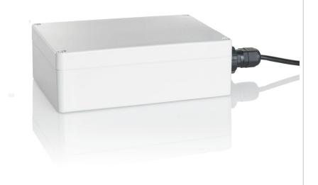
The 30MHz gateway is the central access point for network connectivity in the 30MHz Smart Sensing Toolkit. In its mobile version, the gateway comes equipped with a 3G modem, guaranteeing network access even in the most remote locations, without a fixed internet connection or power supply.
